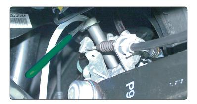
Special brake bleeder wrench for the actuation of bleeder screws. Saves the disassemble and reassemble of the wheels.
