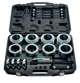
Sleeves outer diameter from: 84 - 122 mm 3 -11/32" - 4-13/16"
